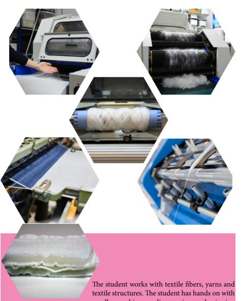
textile structures. The student has hands on with needle punching, carding, roving, and spinning processes in the Advanced Fibre and Yarn Technology course. The student learns 3D knitting (flat, circular, warp), 3D weaving as well as complex structures (braiding and narrow textiles), and advanced nonwovens in the Advanced Textile Structures course.
